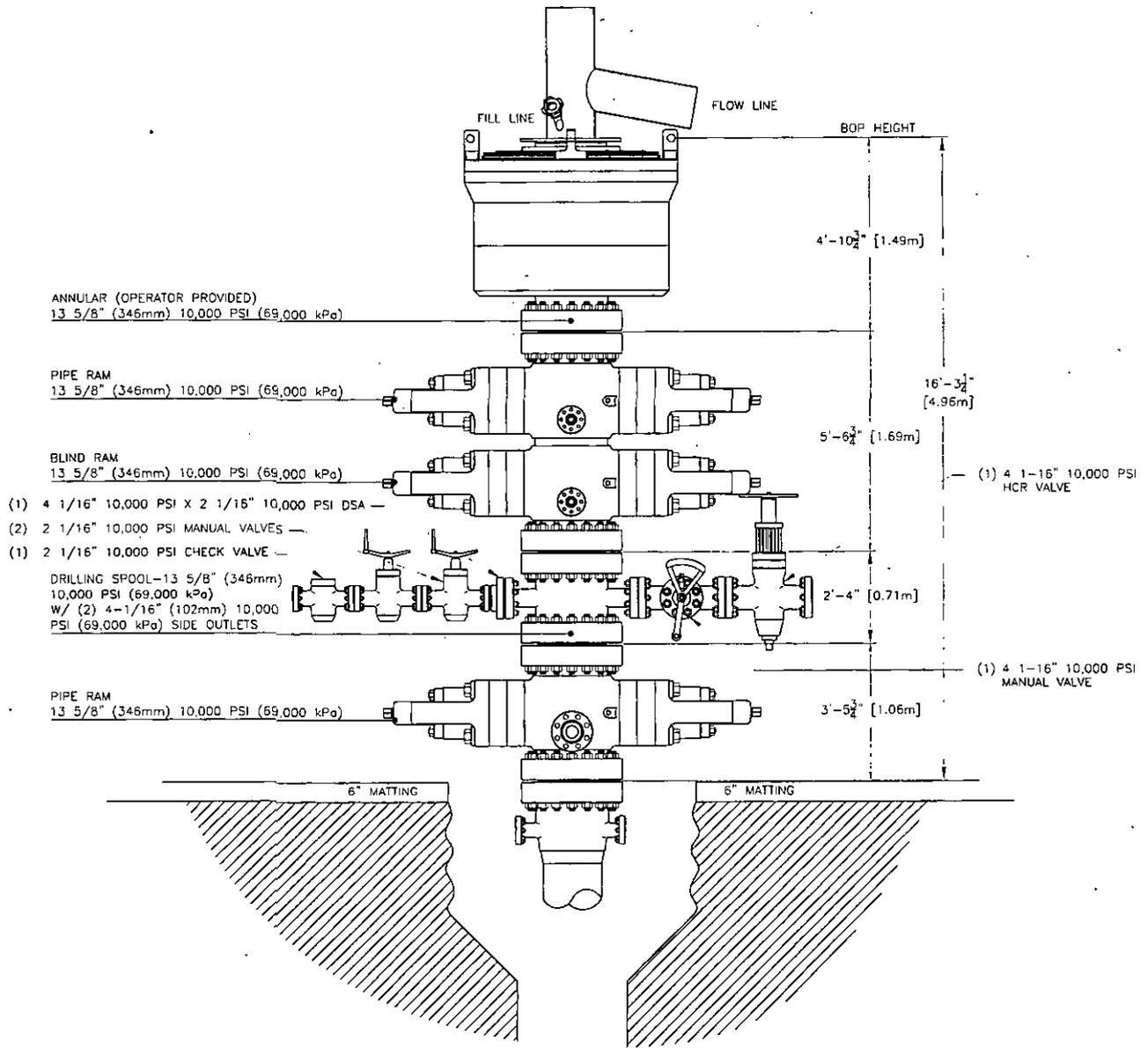
NOTE: CASING BOWL SET AT MATTING LEVEL AND 1/2" ALLOWANCE FOR RING GASKET GAP.
