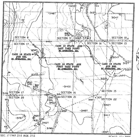
SEC. 17 TWP. 23-S RGE, 27-E SURVEY: N.M.P.M. CQUNTY: EDDY DESCRIPTION: 1650' FNL & 240' FEL ELEVATION: 3164' OPERATOR: B.C. OPERATING, INC. LEASE: CASS 16 STATE U.S.G.S. TOPOGRAPHIC MAP: OTIS, N.M. SCALE: 1" = 2000' CONTOUR INTERVAL = 5'
