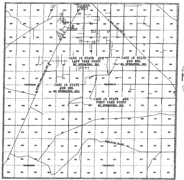
SEC. 17 TWP. 23-S RGE. 27-E SURVEY: N.M.P.M. COUNTY: EDDY DESCRIPTION: 1650' FNL & 240' FEL ELEVATION: 3164' OPERATOR: B.C. OPERATING, INC. LEASE: CASS 16 STATE U.S.G.S. TOPOGRAPHIC MAP: OTIS, N.M. SCALE: 1" = 2 MILES
