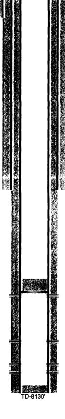
17-1/2" hole @ 572' 13-3/8" csg @ 572' w/ 700sx-TOC-Surf-Circ
