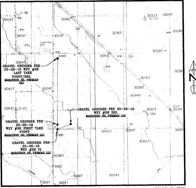
SEC. 18 TWP. 23-S RGE. 28-E SURVEY: N.M.P.M. COUNTY: EDDY DESCRIPTION: 353' FSL & 1265' FWL ELEVATION: 3080' OPERATOR: MARATHON OIL PERMIAN LLC LEASE: GRAVEL GRINDER FEE 23-28-18 U.S.G.S. TOPOGRAPHIC MAP: OTIS, N.M. SCALE: 1" = 2000' CONTOUR INTERVAL = 5'
