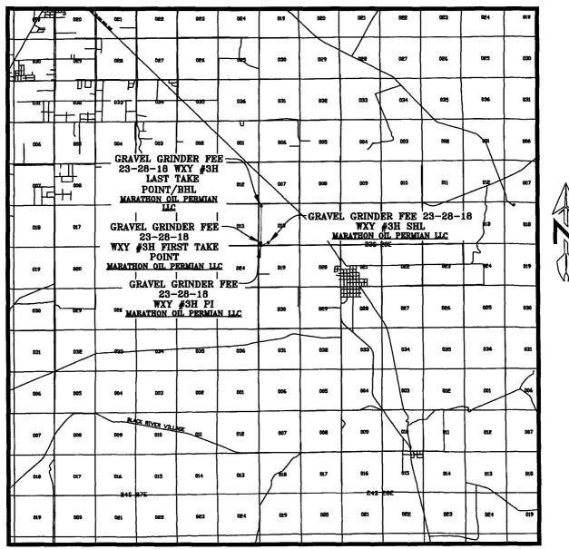
SEC. 18 TWP. 23-S RGE. 28-E SURVEY: N.M.P.M. COUNTY: EDDY DESCRIPTION: 353' FSL & 1265' FWL ELEVATION: 3080' OPERATOR: MARATHON OIL PERMIAN LLC LEASE: GRAVEL GRINDER FEE 23-28-18 U.S.G.S. TOPOGRAPHIC MAP: OTIS, N.M. SCALE: 1" = 2 MILES
