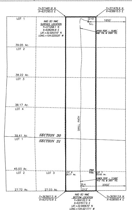
BOREPATH SHOWN HEREON IS BASED ON DIRECTIONAL SURVEY REPORT PROVIDED BY CONCID FOR THE COPPERHEAD 31 FEDERAL COM \$21H SUPPLIED TO HARCROW SURVEYING, LLC ON AUGUST 30, 2017.
