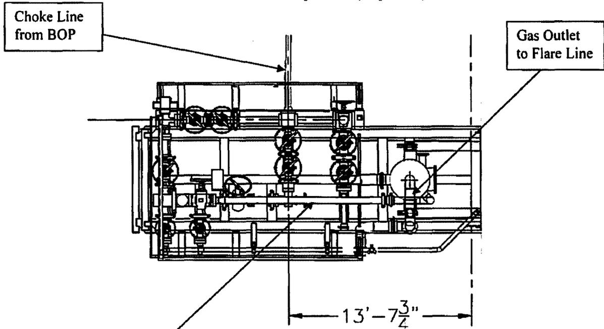
**Choke Manifold – Gas Separator (Side View)**
