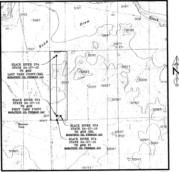
SEC. 15 TWP. 24-S RGE. 27-E SURVEY: N.M.P.M. COUNTY: EDDY DESCRIPTION: 321' FSL & 797' FWL ELEVATION: 3,222' OPERATOR: MARATHON OIL PERMIAN LLC LEASE: BLACK RIVER 374 STATE 24-27-15 U.S.G.S. TOPOGRAPHIC MAP: BOND DRAW, N.M. SCALE: 1" = 2000' CONTOUR INTERVAL = 10'
