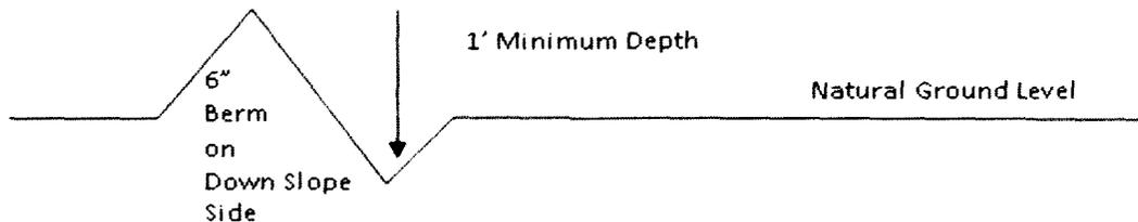
All lead-off ditches shall be graded to drain water with a 1 percent minimum to 3 percent maximum ditch slope. The spacing interval are variable for lead-off ditches and shall be determined according to the formula for spacing intervals of lead-off ditches, but may be amended depending upon existing soil types and centerline road slope (in %);
