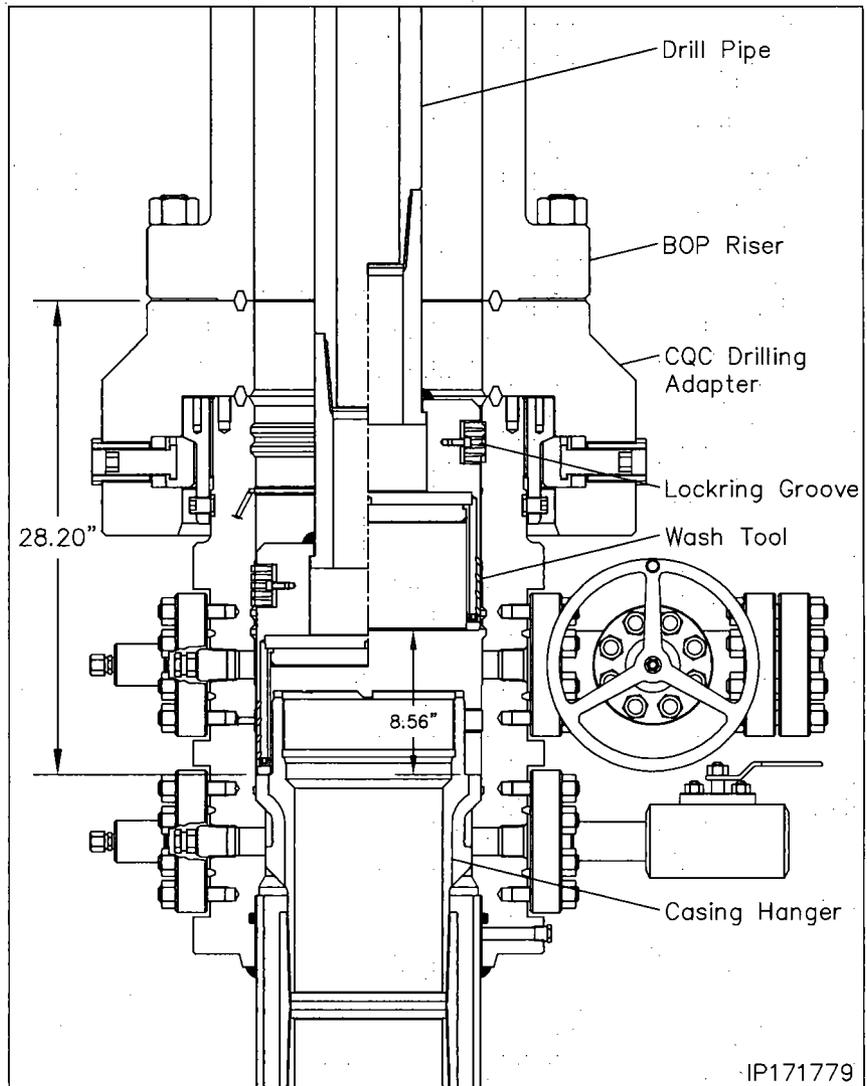
11. Reengage the pump and fully wash the inside of the wellhead and the entire BOP one additional cycle ensuring the stopping point is with the wash tool resting on top of the hanger flutes.
