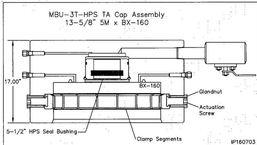
2. Thoroughly clean the top of the MBU-3T housing, thread hub, and the mating seal surfaces of the TA Cap.
