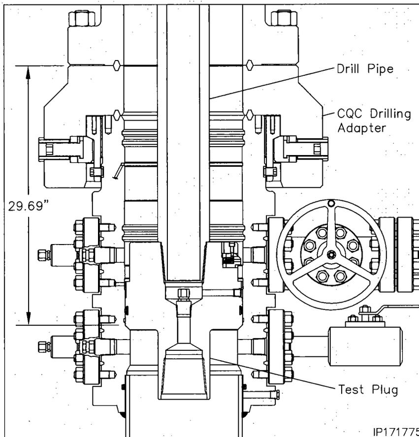
9. Remove as much fluid as possible from the BOP stack and the retrieve the test plug with a straight vertical lift.
