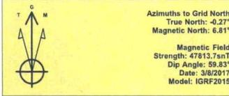
To convert a Magnetic Direction to a Grid Direction, Add 6.82°
