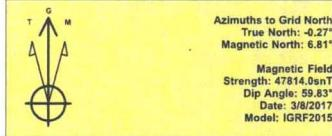
To convert a Magnetic Direction to a Grid Direction, Add 6.81°
