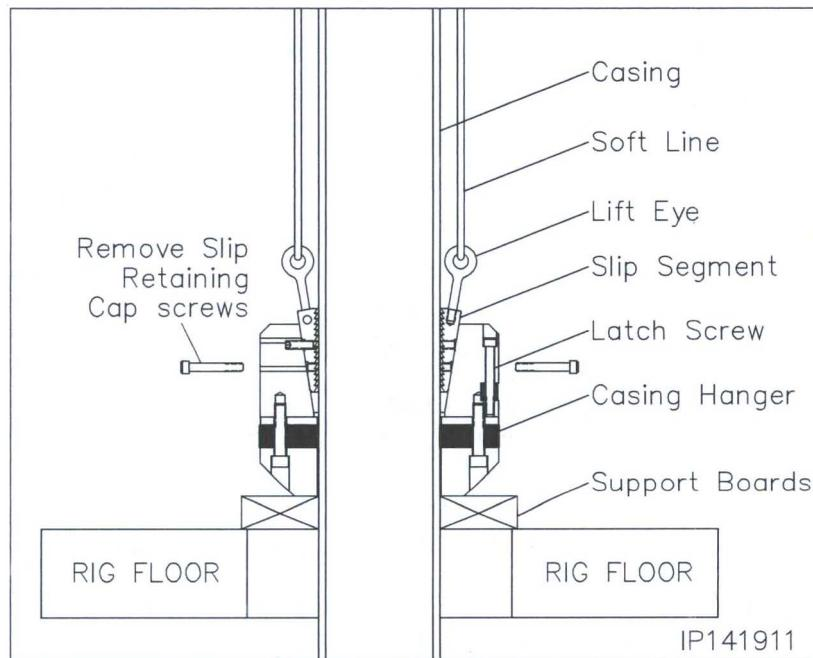
12. Slide the two hanger halves together ensuring the slip guide pins properly engage the opposing hanger half.
