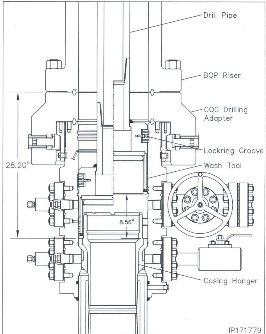
11. Reengage the pump and fully wash the inside of the wellhead and the entire BOP one additional cycle ensuring the stopping point is with the was tool resting on top of the hanger flutes.
