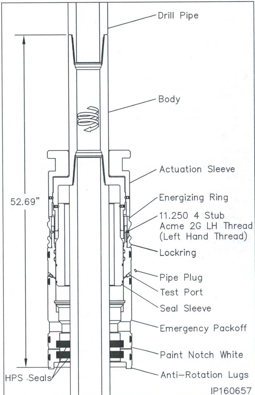
17. Using a straight edge positioned vertically and centered on the anti-rotation lug on the bottom of the packoff, place a white paint mark up the side of the packoff in line with the lug.
