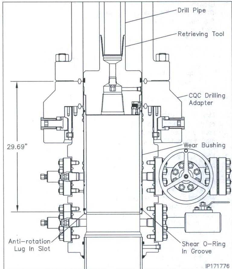
9. Remove the tool from the Wear Bushing by rotating the drill pipe counter clockwise (left) 1/4 turn and lifting straight up.
