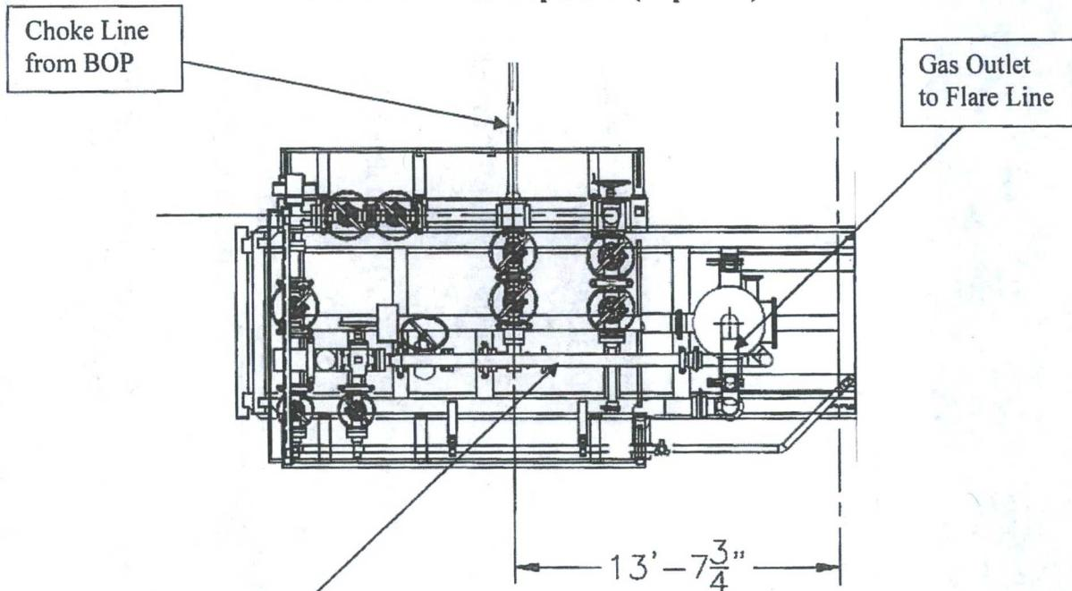
**Choke Manifold – Gas Separator (Side View)**
