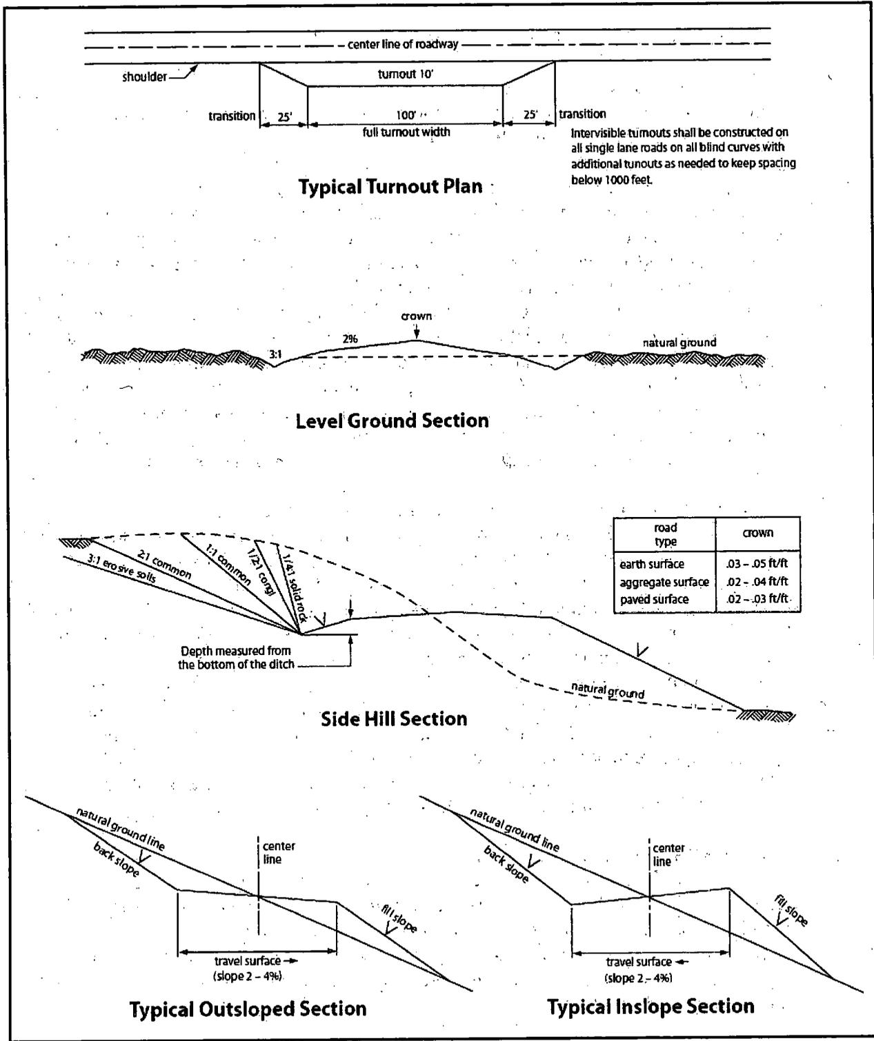
Figure 1. Cross-sections and plans for typical road sections representative of BLM resource or F5 local and higher-class roads.
