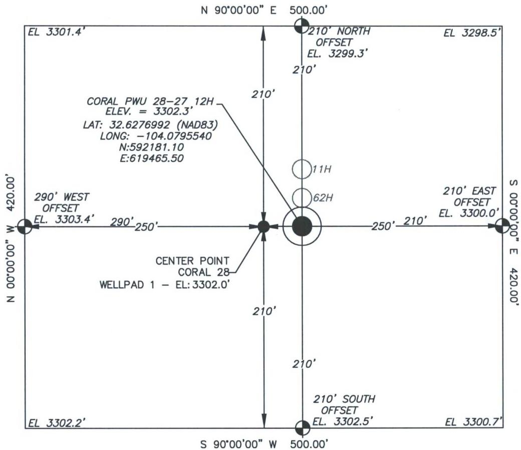
Note: All bearings recited herein are based on the New Mexico State Plane Coordinate System, NAD 83, New Mexico East Zone 3001, US Survey Feet, all distances are grid.
