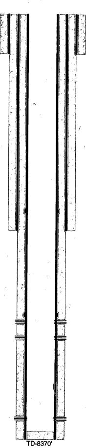
17-1/2" hole @ 803' 13-3/8" csg @ 803' w/ 950sx-TOC-Surf-Circ
