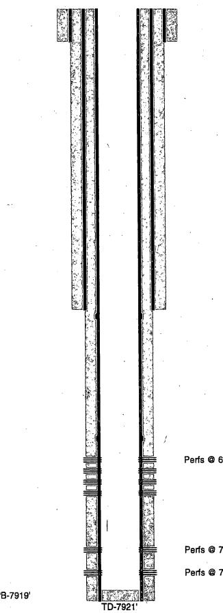
14-3/4" hole @ 428' 11-3/4" csg @ 428' w/ 350sx-TOC-Surf-Circ
