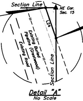
END OF PROPOSED SWD PIPELINE RIGHT-OF-WAY ON STATE OF NEW MEXICO LANDS IN SEC. 15 (At Section Line)
