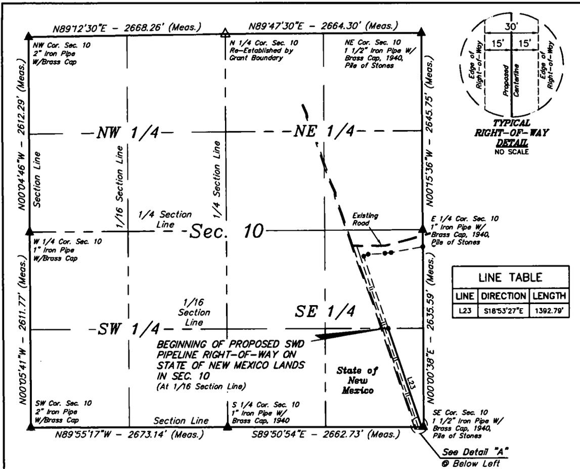
END OF PROPOSED SWD PIPELINE RIGHT-OF-WAY ON STATE OF NEW MEXICO LANDS IN SEC. 10 (At Section Line)
