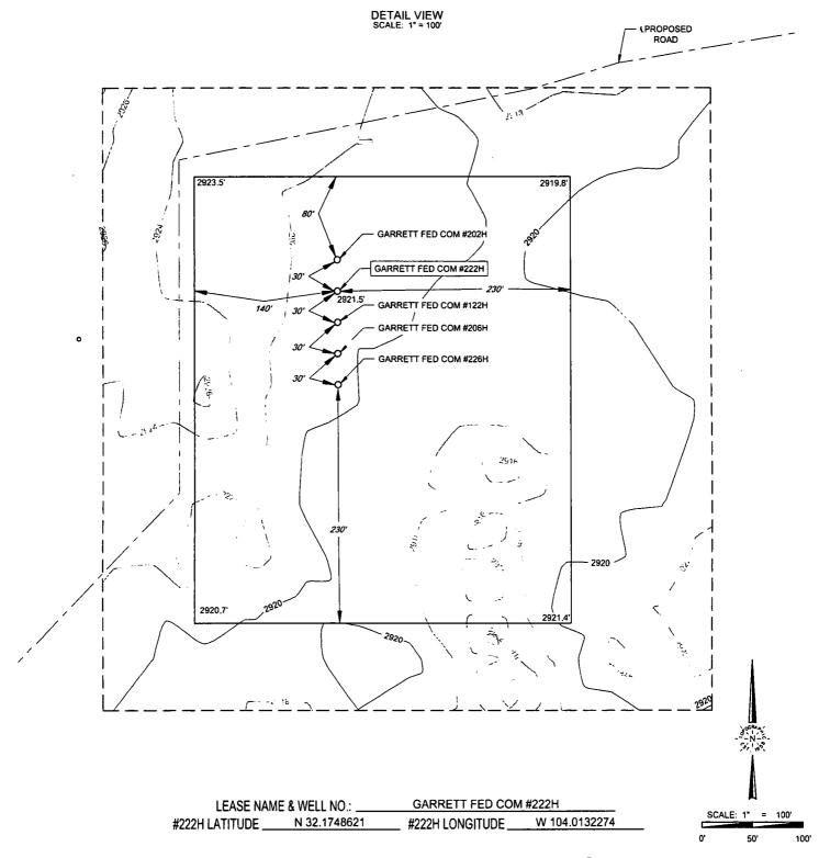
ALL BEARINGS, DISTANCES, AND COORDINATE VALUES CONTAINED HEREON ARE GRID BASED UPON THE NEW MEXICO COORDINATE SYSTEM OF 1983, EAST ZONE, U.S. SURVEY FEET.
