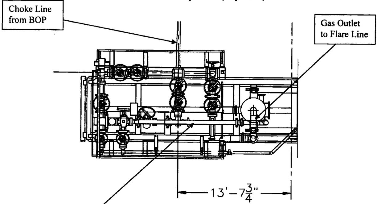
**Choke Manifold – Gas Separator (Side View)**
