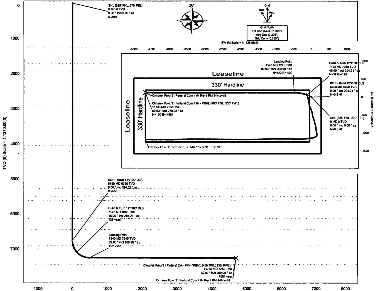
Vertical Section (ft) Azim = 269.98° Scale = 1:1370.00(ft) Origin = 0N/-S, 0E/-W
