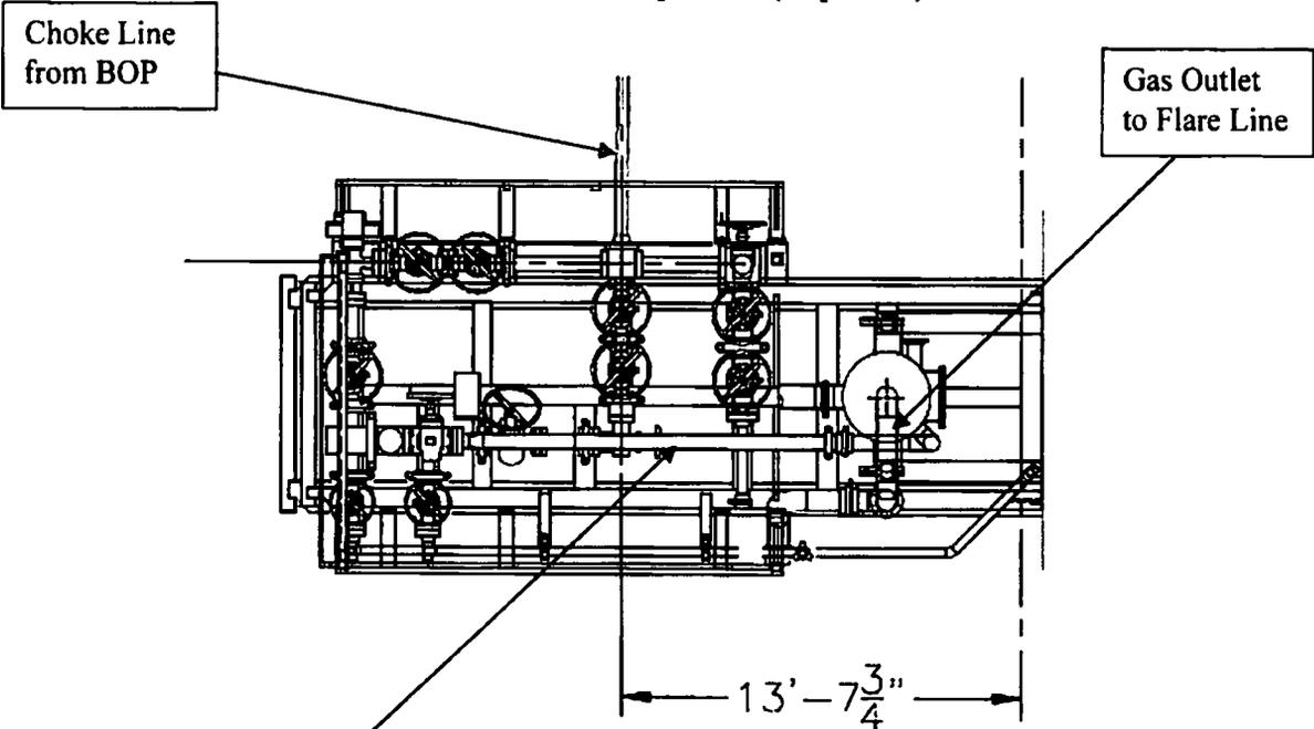
**Choke Manifold – Gas Separator (Side View)**
