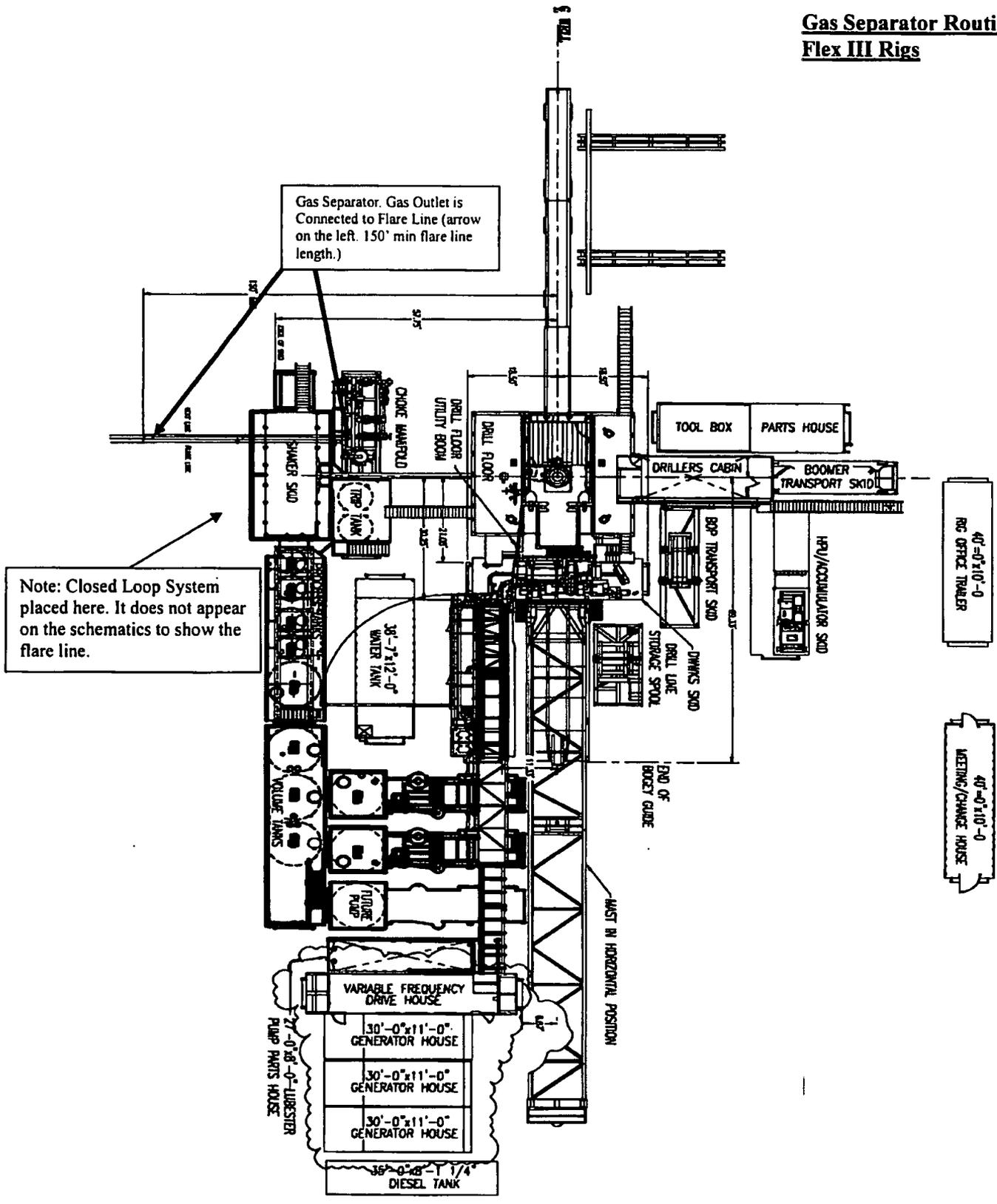
**Choke Manifold – Gas Separator (Top View)**
