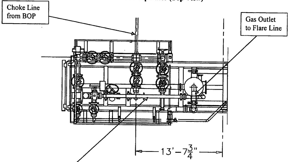
**Choke Manifold – Gas Separator (Side View)**
