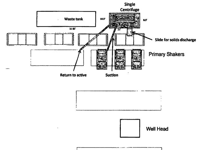
Oxy Single Centrifuge Closed Loop System – New Mexico Flex III May 28, 2013
