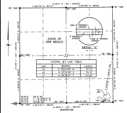
A strip of land 30 feet wide, being 250.11 feet or 15.158 rods in length, lying in Section 32, Township 24 South, Range 30 East, N. M. P. M., Eddy County, New Mexico, being 15 feet left and 15 feet right of the following described survey of a centerline across State of New Mexico land:
