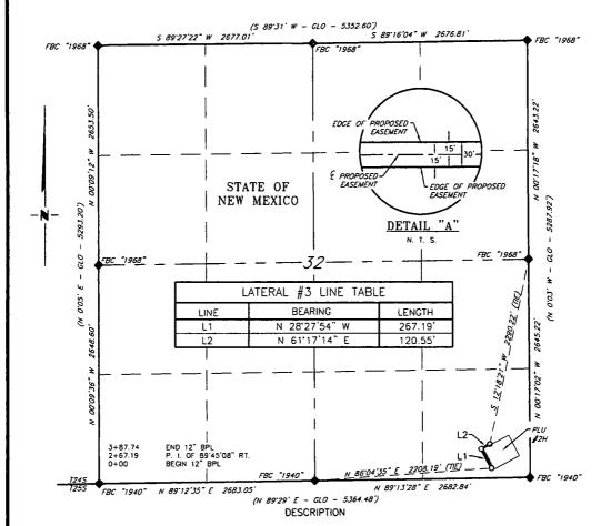
A strip of land 30 feet wide, being 387.74 feet or 23.499 rods in length, lying in Section 32, Township 24 South, Range 30 East, N. M. P. M., Eddy County, New Mexico, being 15 feet left and 15 feet right of the following described survey of a centerline across State of New Mexico land:
