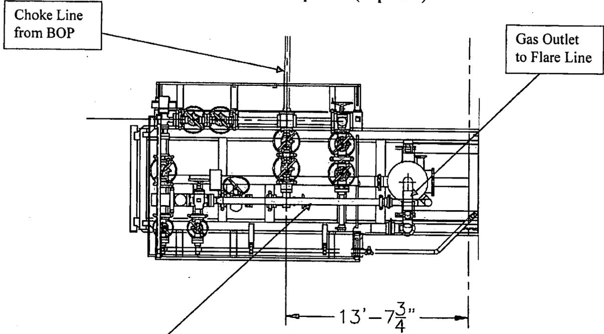
**Choke Manifold – Gas Separator (Side View)**
