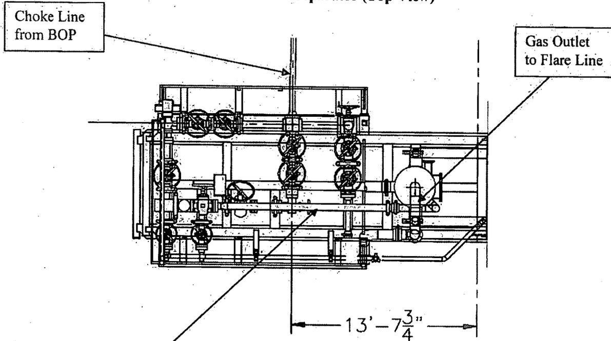
**Choke Manifold – Gas Separator (Side View)**
