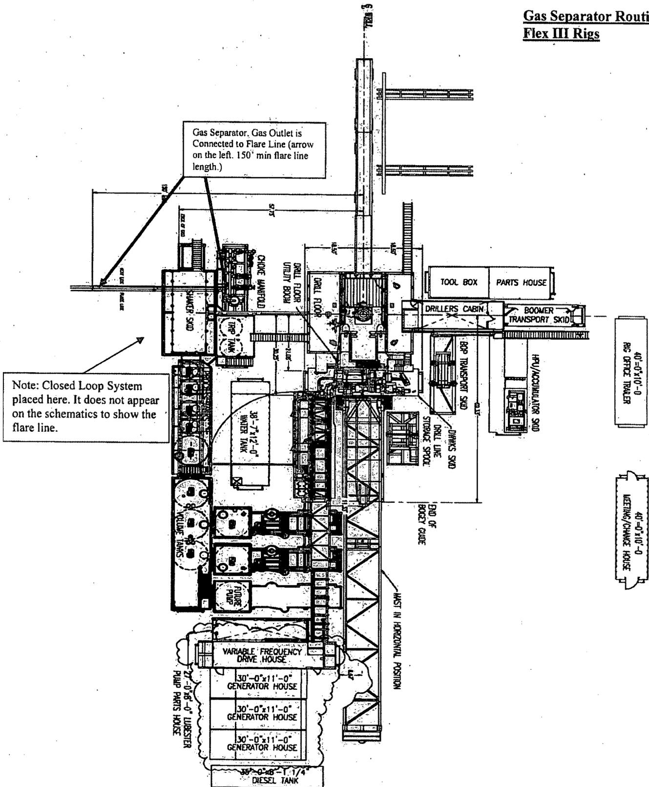
**Choke Manifold – Gas Separator (Top View)**
