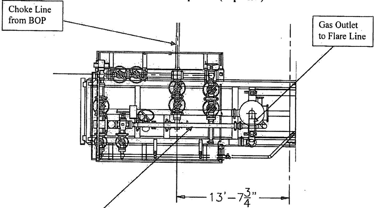
**Choke Manifold – Gas Separator (Side View)**
