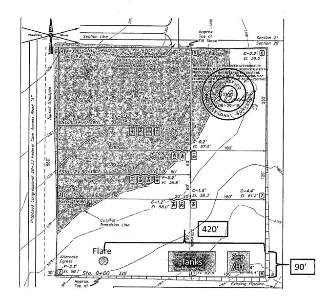
\*\*Must maintain min. 100' from equipment to wellhead. Flare must be 150'
