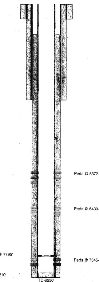
17-1/2" hole @ 535' 13-3/8" csg @ 535' w/ 950sx-TOC-Surf-Circ-1"
