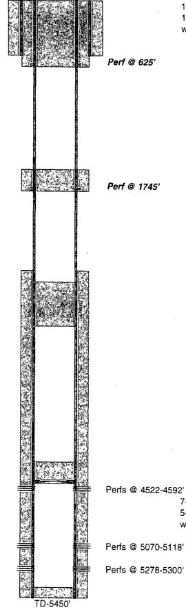
14-3/4" hole @ 575' 10-3/4" csg @ 575' w/ 600sx-TOC-Surf-Circ
