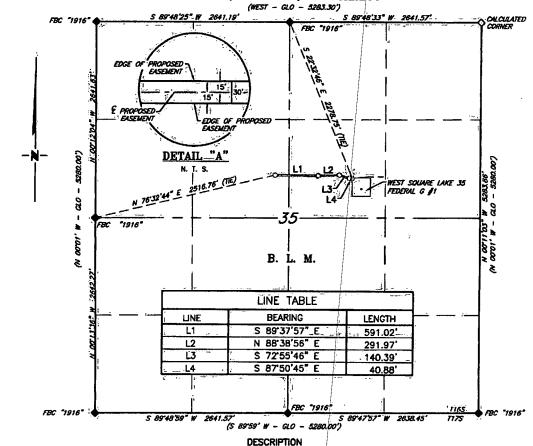
A strip of land 30 feet wide, being 1,064.26 feet or 64.501 rods in length, lying in Section 35, Township 16 South, Range 30 East, N. M. P. M., Eddy County, New Mexico, being 15 feet left and 15 feet right of the following described survey of a centerline across B. L. M. land:
