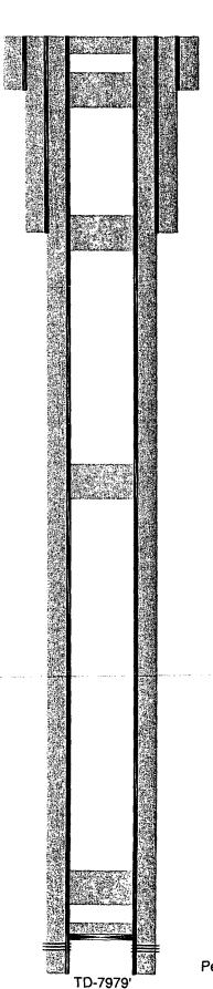
17-1/2" hole @ 400' 13-3/8" csg @ 400' w/400sx-TOC-Surf-Circ
