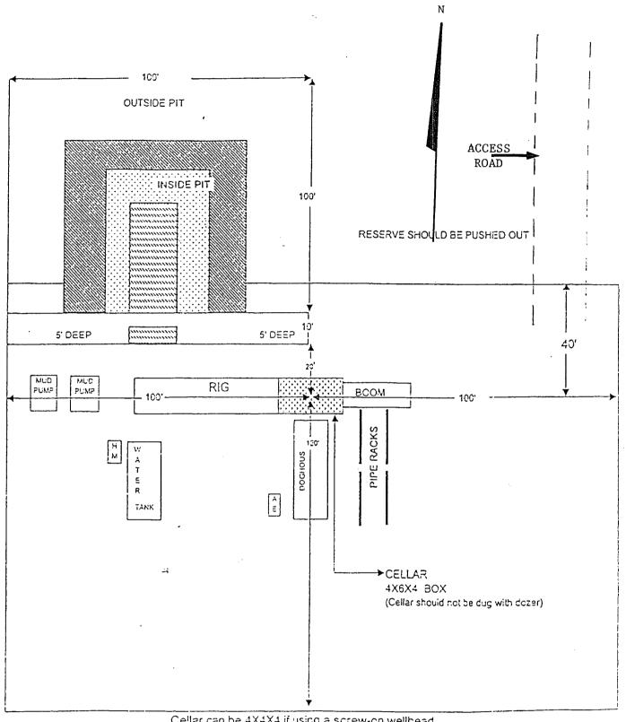
Cellar can be 4X4X4 if using a screw-on wellhead Working Pits dug 5' below ground level
