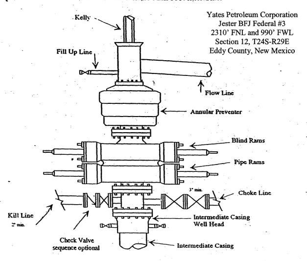
Typical 3,000 psi choke manifold assembly with at least these minimum features
