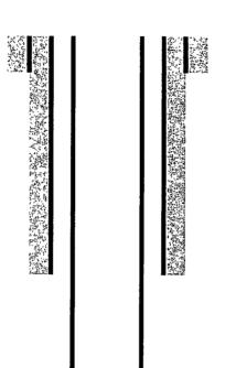
17-1/2" hole @ 325' 13-3/8" csg @ 325' w/380sx-TOC-Surf-Circ
