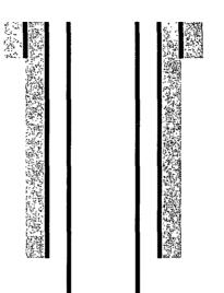
17-1/2" hole @ 325' 13-3/8" csg @ 325' w/380sx-TOC-Surf-Circ
