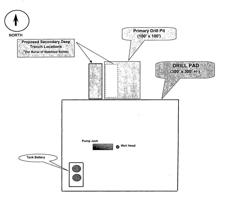
Note: Location of solids burial trench will be determined in the field based on site conditions, i.e. (terrain slope, vegetatation, etc.)
