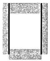
12-1/4" hole @ 1512' 9-5/8" csg @ 1512' w/ 1140sx-TOC-Surf-Circ
