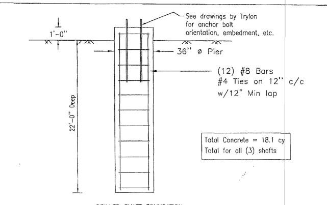
DRILLED SHAFT FOUNDATION
