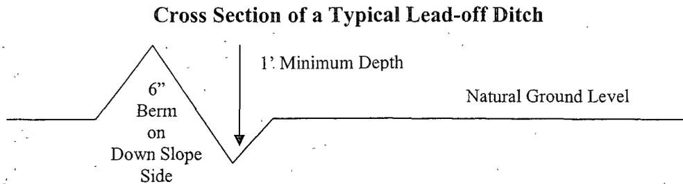
All lead-off ditches shall be graded to drain water with a 1 percent minimum to 3 percent maximum ditch slope. The spacing interval are variable for lead-off ditches and shall be determined according to the formula for spacing intervals of lead-off ditches, but may be amended depending upon existing soil types and centerline road slope (in %);
