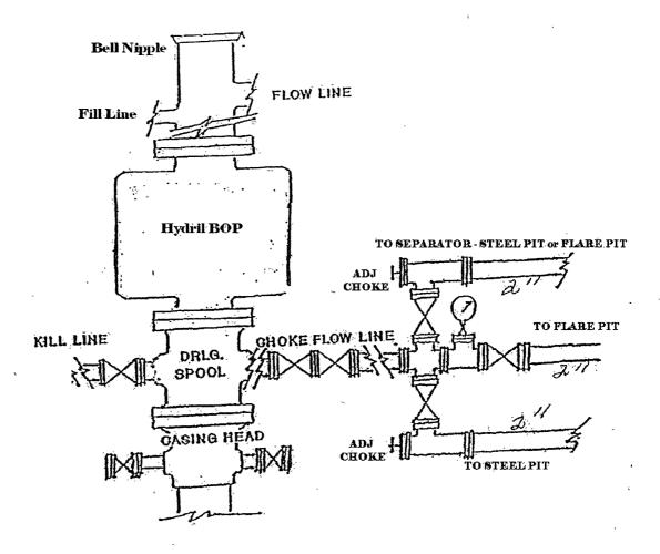
Flare Line 150 ft From Wellhead. Ignition By Remote Source
