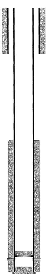
14-3/4" hole @ 1500' 9-5/8" csg @ 1500' w/ 1380sx-TOC-Surf-Circ
