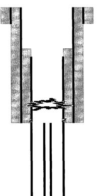
17-1/2" hole @ 405' 13-3/8" csg @ 405' w/450sx-TOC-Surf-Circ
