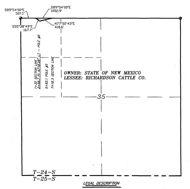
A STRIP OF LAND 30.0 FEET WIDE, LOCATED IN SECTION 35, TOWNSHIP 24 SOUTH, RANGE 30 EAST, N.M.P.M., EDDY COUNTY, NEW MEXICO AND BEING 15.0 FEET LEFT AND RIGHT OF THE FOLLOWING DESCRIBED CENTERLINE SURVEY.
