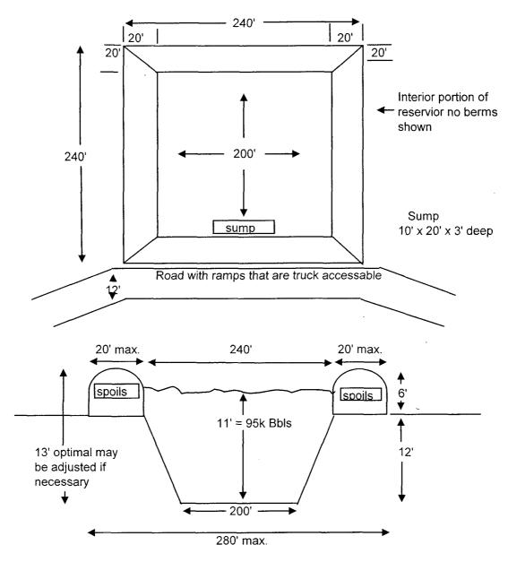
Spoil piles= 3 sides will normally be narrow and the fourth side will include the road and access to the sump.
