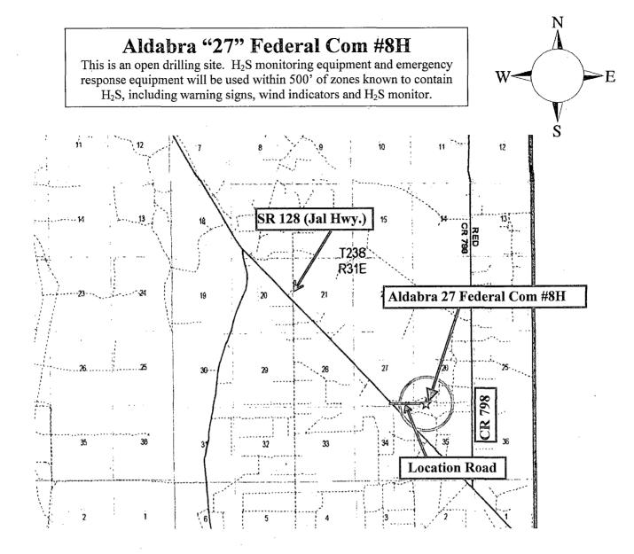
Assumed 100 ppm  $\mathbb{ROE} = 3000^\circ$  (Radius of Exposure) 100 ppm H2S concentration shall trigger activation of this plan.
