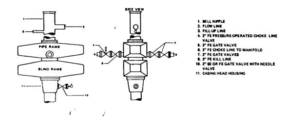
Figure 7-10. Standard Hydraulic Blowout Preventer Assembly (2 M or 3 M Working Pressure) Alternative 3 (without Drilling Spool)
