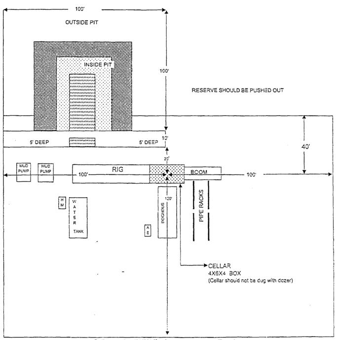
Cellar can be 4X4X4 if using a screw-on wellhead Working Pits dug 5' below ground level
