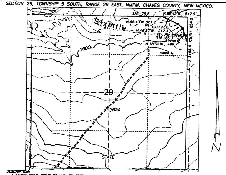
A LEASE ROAD RIGHT OF WAY 30 FEET WIDE, BEING 15 FEET TO THE LEFT AND RIGHT OF THE FOLLOWING DESCRIBED SURVEY CENTERLINE:
