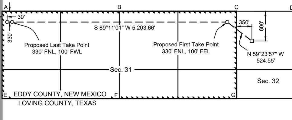
The diagram shows a well location plat across sections 31 and 32. The well is located in Section 31, 330' from the north line and 100' from the east line. A proposed first take point is 330' from the north line and 100' from the east line. A proposed last take point is 330' from the north line and 100' from the west line. The well is 350' from the north line and 600' from the east line. The diagram also shows the boundary between Eddy County, New Mexico and Loving County, Texas.
