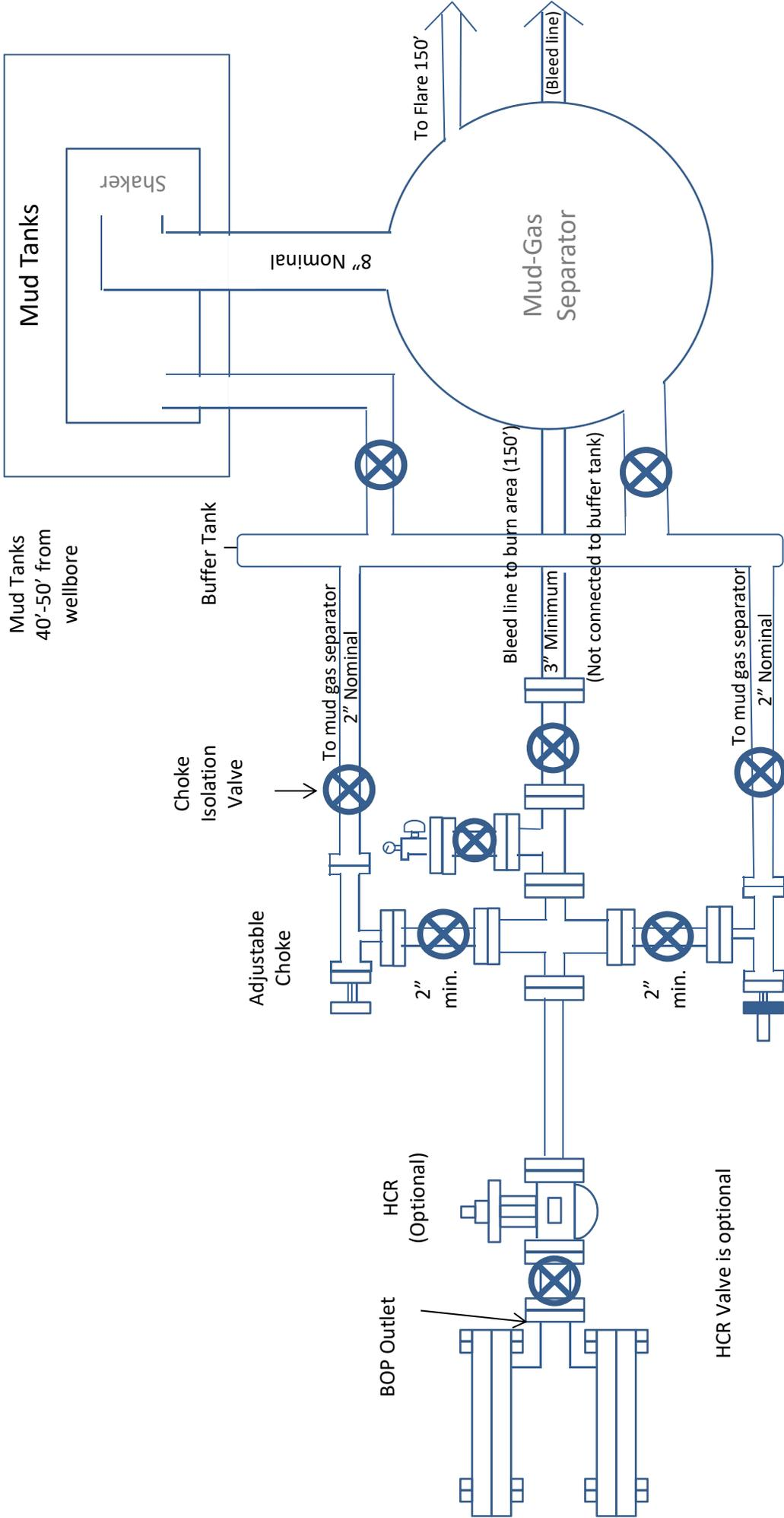
2M & 3M Choke Manifold Diagram
